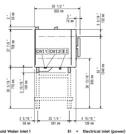
Cold Water inlet 1 CWI2 Cold Water Inlet 2 D Drain
